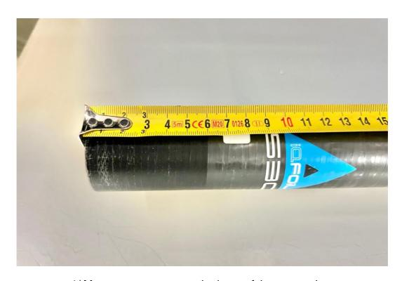
1/ Measurement starts at the base of the top section.
