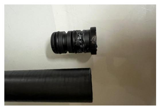
3/ Plastic top cup can be removed and installed on the new top. The plastic cup top keeps the water out of the mast
