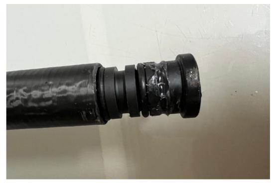
4/ Plastic cup can be fitted easily on the top section. Any kind of glue or tape can be applied to guarantee that it doesn't come off.
